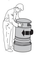
Lift bin body over liner and drop onto plinth to lock.
